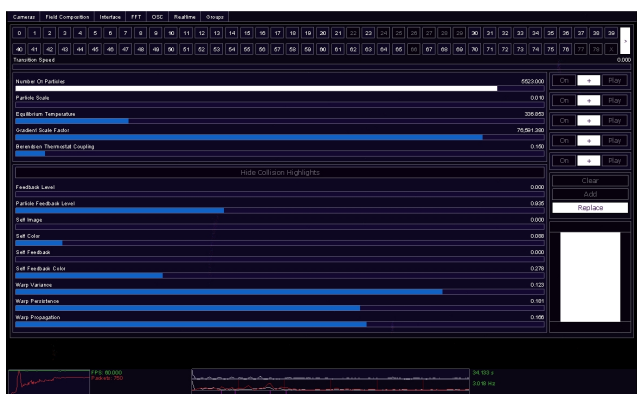
Figure 7: primary interface screen of the 7-tab dS GUI. The sliders and buttons allow control over a range of physics and graphics parameters. The graphs on the bottom relate to the real-time vibrational spectrum of the atomic dynamics, and the rows of numbers at the top allow the dS operator to rapidly save and access a range of dS states
