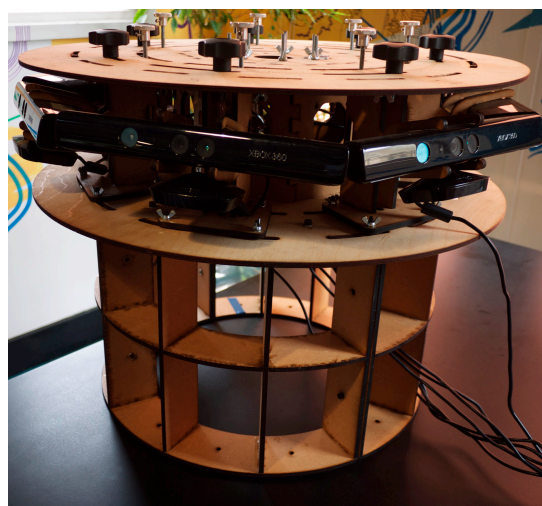
Figure 6: Our custom-built 360° optical mount which houses seven depth sensors in a circular arrangement.
