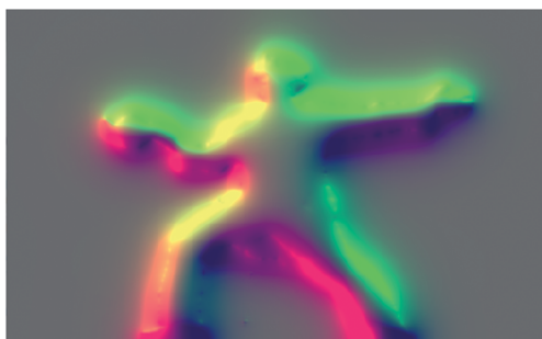
Fig. 1 Force topology map of the human form. The intensity of each color is related to the magnitude of the local force vector on the depth image. Color choice has been selected to effectively illustrate depth. Grey corresponds to a gradient of zero.
