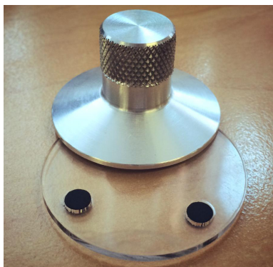
Figure 6. Components of the current prototype widget utilising conductive plastic contact points.
